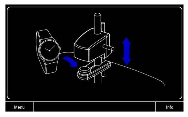
Move the measuring head vertically by simultaneously pulling on the lever and raising or lowering the measuring head as shown in the picture below.
