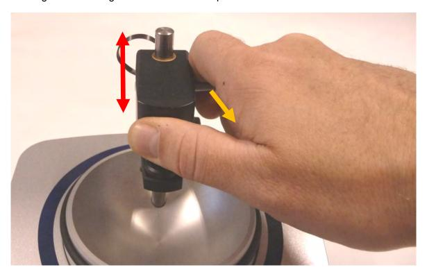
If the watch does not fit correctly into the space, you can also move the watch support vertically by loosening the screw on the side.
