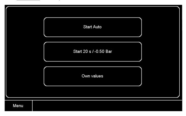
Now select the Measurement parameters by touching and dragging the controller that you want to adjust. Once you have set up the values to suit your requirements, press Start to begin measurement. The values you have selected are now saved for future measurements on the middle button in the Start menu.
